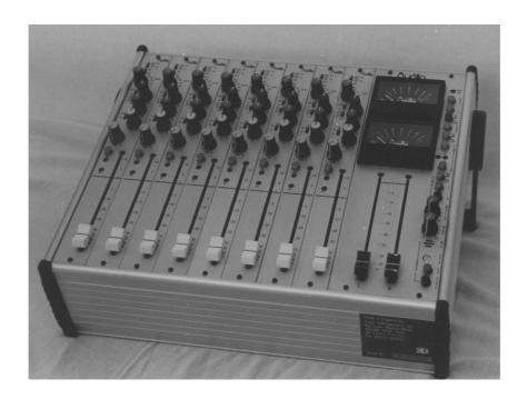
Radical change and PICO have proved to be uneasy bedfellows: never a matinée idol and denied its *dulce et decorum* death, AD145 has now been repackaged in the 140 series metalwork - thereby reducing its size and weight. Facilities remain largely unchanged: internally, the microphone amplifier has been replaced with the one designed for AD146 and externally, the mono return is now in stereo form. Now designated AD245, shall we have PICO - like the poor - always with us?
